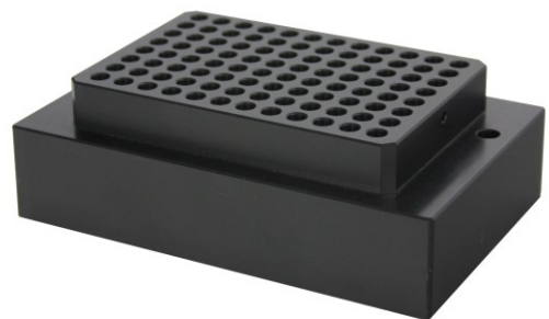
L150 x W95 x H50mm, black anodised aluminium
